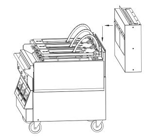
8. Roll grill under hood. Grill must be level front to back, side to side and diagonally. Adjust casters accordingly to obtain final level.
